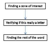
Fig. 4. Three steps in text detection algorithm [14]
