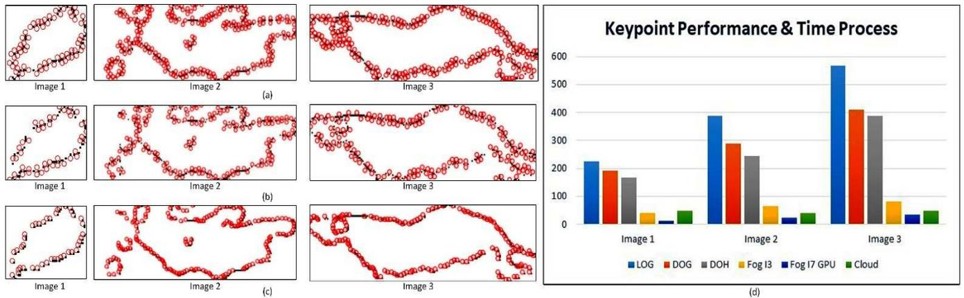
Fig. 4 (a) Blob detection using LoG; (b) Blob detection using DoG; (c) Blob detection using DoH; (d) Key performance blob detection and time process on server fog and server cloud
