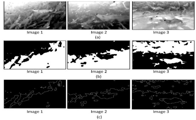
Fig. 2 (a) Grayscale image; (b) Thresholding image; (c) Edge detection of shrimp image data underwater
