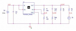
Fig. 3 TPS76301 test circuit
