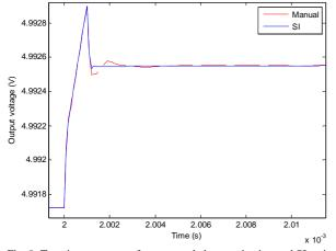
Fig. 9 Transient responses from manual characterization and SI-estimated model simulation for ESR of 10  $\Omega$  and load current of 50 mA
