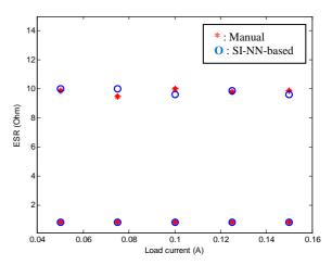
Fig. 8 Comparison of critical ESR on the failure region boundaries between manual and SI-NN-based VR characterization
