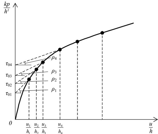
Fig. 2 Graphical determination of the limiting shear stress of a capillary-porous material
