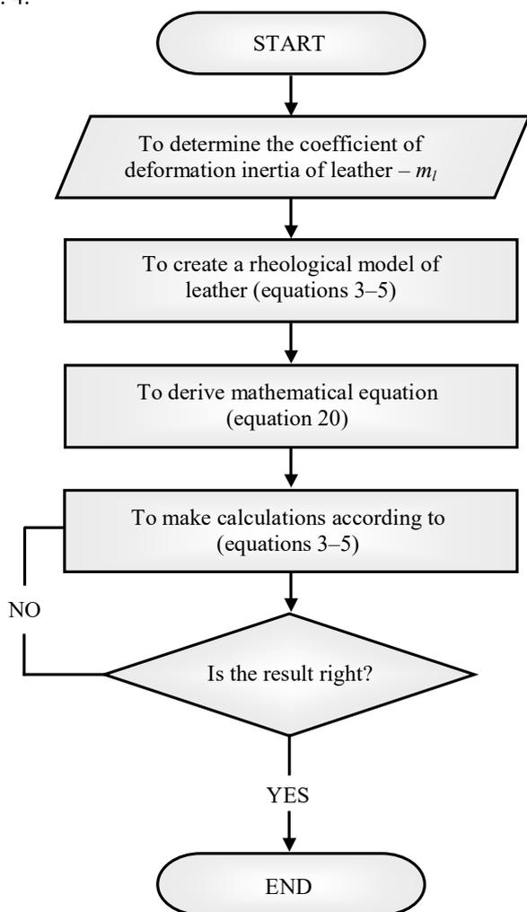
Fig. 4 Block diagram of the proposed method for improving the rheological model of leather
