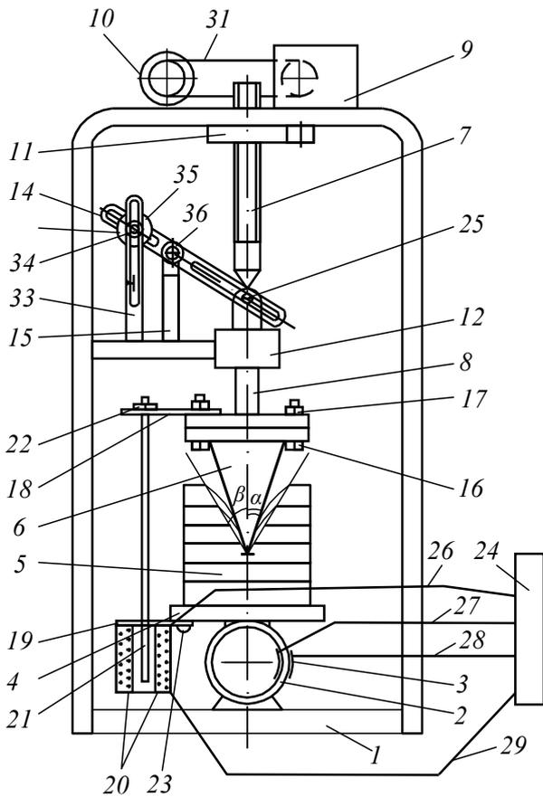
Fig. 1 Scheme of an experimental stand for determining the rheological parameter of a capillary-porous material
