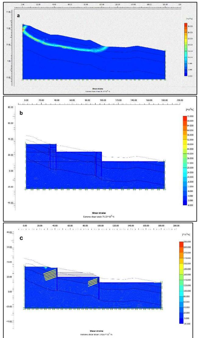
Fig. 6 Analysis of the stability by using FE method (a) FS before excavation (b) FS global of piles cap (c) FS global of piles anchor
