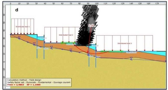
Fig. 9 Analysis of the stability by using LE method a) FS before excavation b) FS global c,d) FS in the critical places of piles cap
