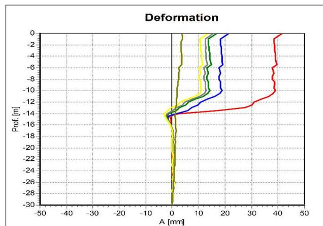
Fig. 5 Horizontal deformation of the soil at the inclinometer (I2 bis)
