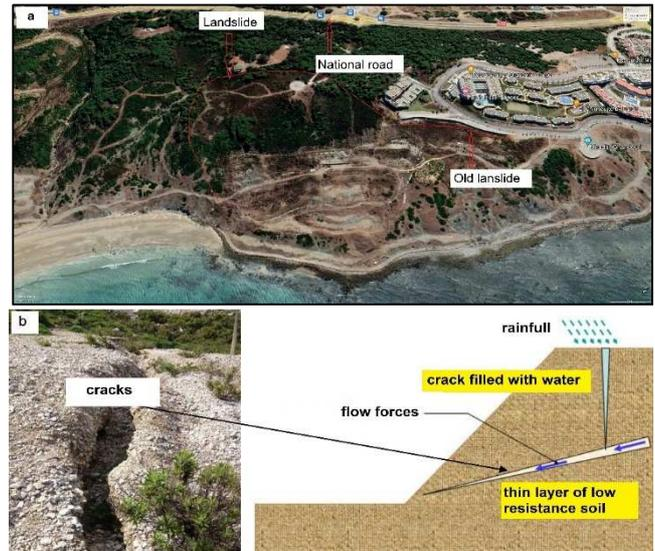
Fig. 3 a) Recent landslide, b) cause of the landslide
