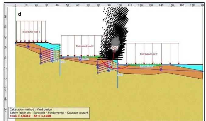
Fig. 8 Analysis of the stability by using LE method a) Engineering geologic profile a-a' b) FS global c,d) FS in the critical places of piles anchor
