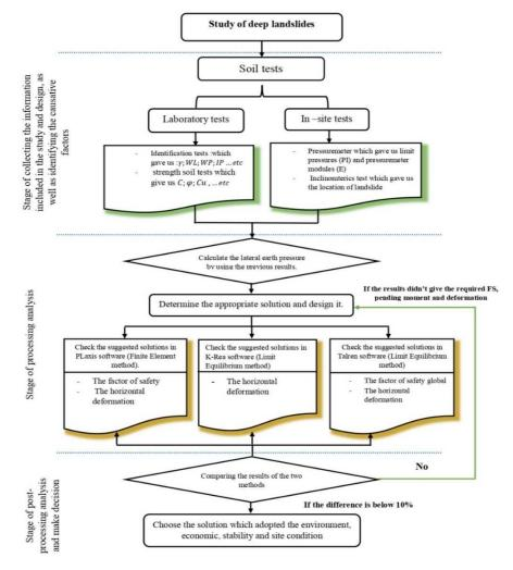
Fig. 5 The flowchart of the proposed methodology used in this research
