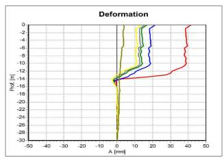
Fig. 5 Horizontal deformation of the soil at the inclinometer (I2 bis)
