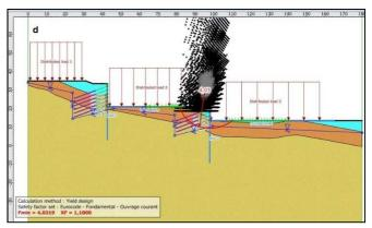
Fig. 8 Analysis of the stability by using LE method a) Engineering geologic profile a-a' b) FS global c,d) FS in the critical places of piles anchor
