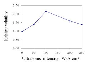
Fig.4 Relative volatility of Chx/ Bz as a function of ultrasonic intensity at frequency of 40 kHz
