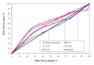
Fig.2 xy- diagram of Chx/ Bz system with different ultrasonic intensities
