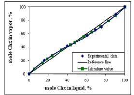
Fig. 1 Equilibrium diagram of Chx - Bz without the presence of ultrasonic wave at atmospheric pressure [•] experimental value [**1**] literature value [12]
