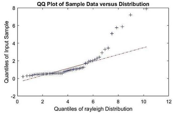
Fig. 1 Q-Q plot for the first unit's data of Mosul Dam.
