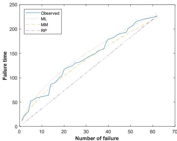
Fig. 4 Plotting the number of failures against  $S_i$  and  $\hat{S}_i$  for the second unit of Mosul Dam.
