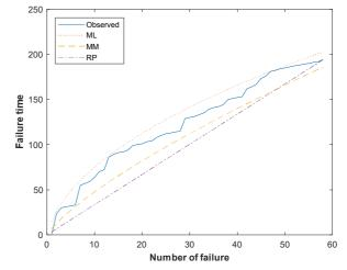
Fig. 3 Plotting the number of failures against  $S_i$  and  $\hat{S}_i$  for the first unit of Mosul Dam.
