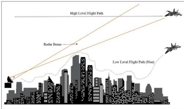
Fig. 1 The below aircraft is flying at the low altitude to avoid Radar detection and recognition
