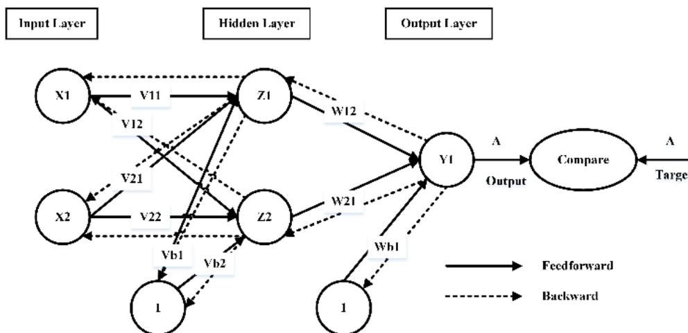
Fig. 3 The architecture of BPNN
