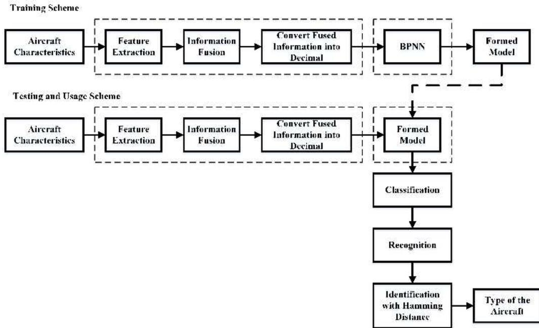
Fig. 4 Detailed model of the system that shows how BPNN generates knowledge
