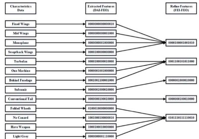
Fig. 5 Utilizing the information fusion to obtain five primary features as the inputs to BPNN
