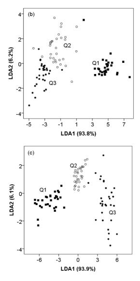
Fig. 11 LDA plot for three quality levels of dried black tea. (a) without heating or treatment I, (b) with unstable heating or treatment II, and (c) with stable heating or treatment III
