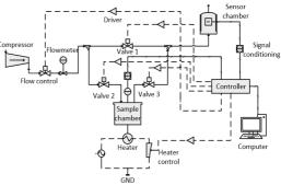
Fig. 1 Schematic diagram of the e-nose system
