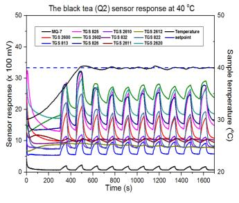
Fig. 7 Sensor responses generated at the set point of 40 °C
