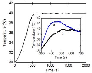
Fig. 5 A typical of the temperature controller performance when the set point is 40 °C. Inset is the time response a) less than 600 s, b) more than 700 s
