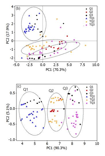
Fig. 10 Score plot of PCA for three quality levels of dried black tea. (a) without heating or treatment I, (b) with unstable heating or treatment II, and (c) with stable heating or treatment III. TQx is the test sample of Qx
