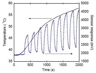
Fig. 6 Increasing the sensor response due to increasing the temperature of the sample
