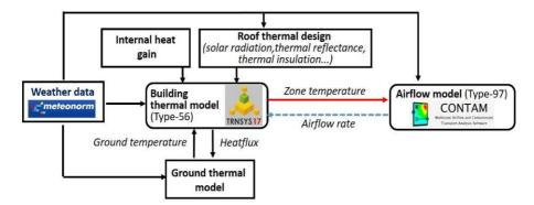
Fig. 3 Coupled simulation model between TRNSYS and CONTAM in the building model [19]
