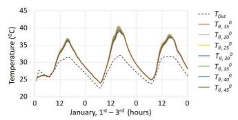
Fig. 5 Air temperature profile in attic zone based on roof slope angle for 3 consecutive days
