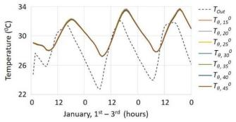
Fig. 6 Operative temperature profile of zone for different roof slope angle for 3 consecutive days
