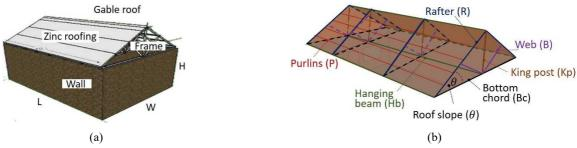
Fig. 1 The prototype of the analyzed building: a. 3D building Presentation, b. Gable roof construction with truss roof framing
