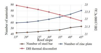
Fig. 7 The effect of the roof slope on the amount of steel rod and galvanized steel plate needed and the value of DH thermal discomfort
