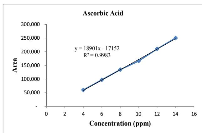
Fig. 1 Vitamin C Standard Curve
