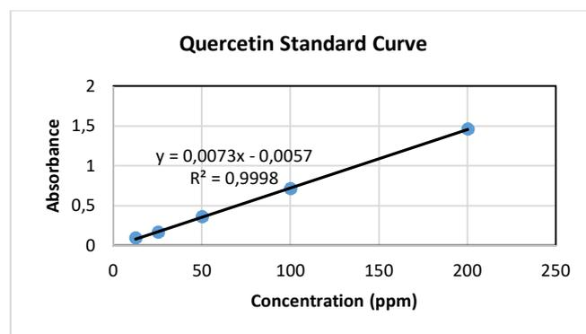
Fig. 3 Quercetin Standard Curve
