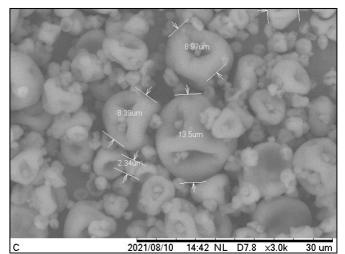
Fig. 4 Microstructure of jack bean tempeh protein isolate with a variation of 160°C inlet air temperature observed using SEM with 3000x magnification
