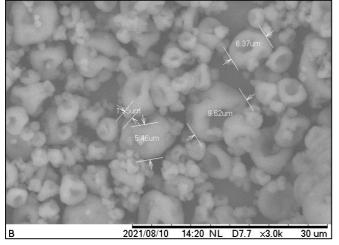
Fig. 3 Microstructure of jack bean tempeh protein isolate with a variation of 150°C inlet air temperature observed using SEM with 3000x magnification
