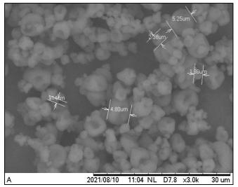
Fig. 2 Microstructure of jack bean tempeh protein isolate with a variation of 140°C inlet air temperature observed using SEM with 3000x magnification
