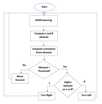
Fig. 3 Collision-avoidance algorithm flowchart [22]
