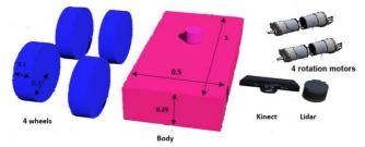
Fig.2 Designed Mobile robot with details in Webots simulator (open-source simulator [21])
