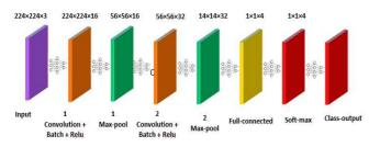
Fig. 6 Twelve layers and a K-NN classifier in CNN localization
