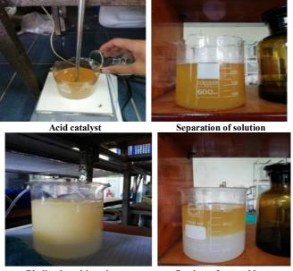
Biodiesel washing phase Product after washing Fig. 1 Synthesis of biodiesel from pangasius fish fat
