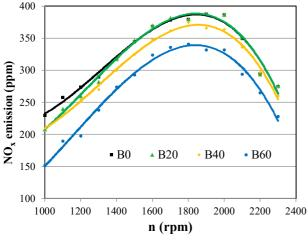
Fig. 7 NO<sub>x</sub> emissions vs engine speed for different biodiesel blends
