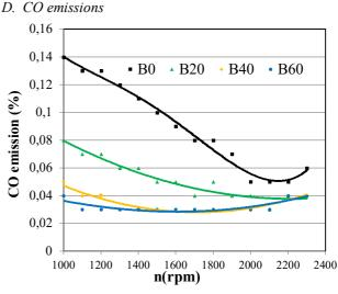
Fig. 6 CO emissions vs engine speed for different biodiesel blends
