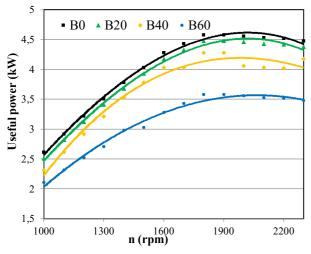
Fig. 4 Useful power vs engine speed for different biodiesel blend ratios
