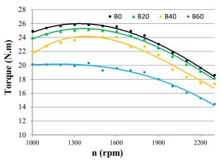
Fig. 3 Torque change with different fuels
