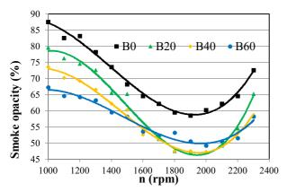
Fig. 10 Smoke opacity vs engine speeds for different biodiesel blend ratios
