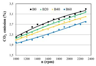
Fig. 9 CO<sub>2</sub> emissions vs engine speed with different biodiesel blends
