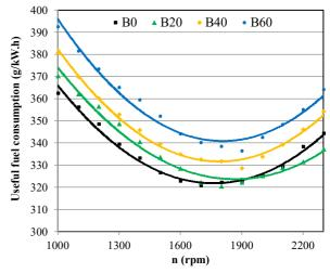
Fig. 5 Useful fuel consumption vs engine speed with different biodiesel blends  $% \left( {{{\left[ {{{\rm{c}}} \right]}}_{{\rm{c}}}}_{{\rm{c}}}} \right)$
