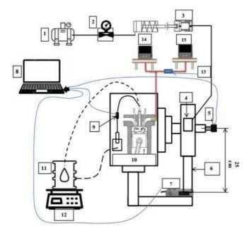
Fig. 2 Experimental layout: (1) compressed air tank, (2) pressure regulator, (3) main pneumatic cylinder, (4) brake cylinder, (5) speed sensor, (6) lever, (7) engine force gauge, (8) computer, (9) pressure sensor, (10) engine, (11) fuel tank, (12) scale, (13) smoke filter, (14) opacimeter OP 160, (15) exhaust analyzer KEG 500
