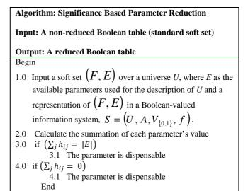
Fig. 2 The algorithm of the significance based parameter reduction
