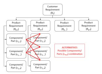
Fig. 1 Relationships between customer requirements and technical product requirements, and the possible combinations of components that meet the requirements
