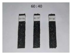
Fig. 12 Weight Fraction Composite 40% (60:40)
