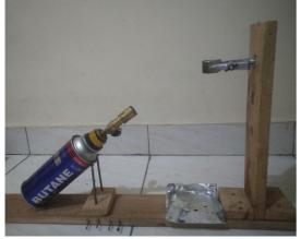
Fig. 5 Fire Resistance Test Equipment
