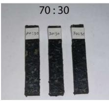
Fig. 11 Weight Fraction Composite 30% (70:30)
