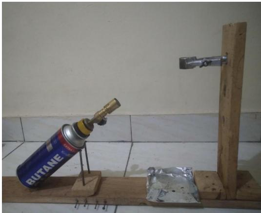
Fig. 5 Fire Resistance Test Equipment
