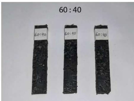
Fig. 12 Weight Fraction Composite 40% (60:40)
