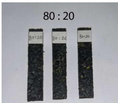
Fig. 10 Weight Fraction Composite 20% (80:20)
