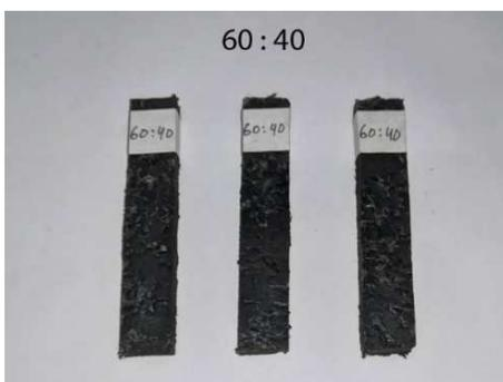
Fig. 12 Weight Fraction Composite 40% (60:40)
