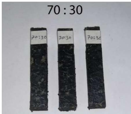
Fig. 11 Weight Fraction Composite 30% (70:30)
