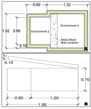
Fig. 4 Dimensions of the test chamber (A) Landscape view and (B) Side View
