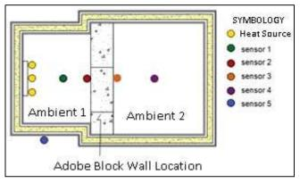
Fig. 7 Location of thermal sensors
