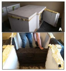
Fig. 5 (A) Acoustic and thermal test chamber, (B) Adobe block wall inside the test chamber
