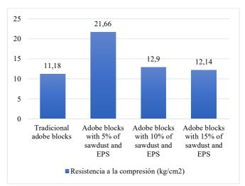
Fig. 3 Average compressive strength (kg/cm2) in blocks with different composition
