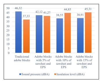
with greater isolation being the more adobe 15% sawdust and EPS with 45.31dBA insulation.
