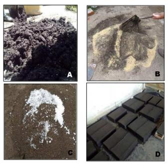
Fig. 1 (A)Sifted land, (B) Adding of sawdust, (C)Adding of EPS, (D) Adobe blocks molding
