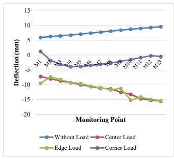
Fig. 9 Plain concrete pavement deflection pattern with swelling pressure
