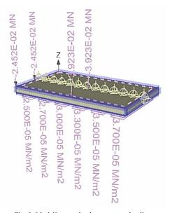
Fig. 8 Modeling results due to corner loading
