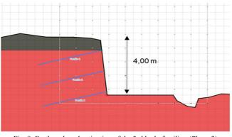
Fig. 8 Earthwork and activation of the 3rd bed of nailing (Phase 3)
