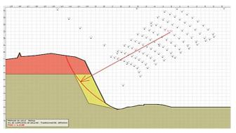
Fig. 5 Result of the stability calculation
