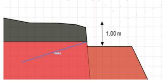
Fig. 6 Earthmoving and activation of the first nailing bed (Phase 1)
