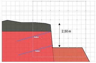
Fig. 7 Earthwork and activation of the 2nd bed of nailing (Phase 2)
