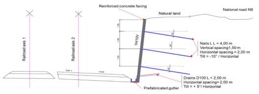
Fig. 10 Characteristics of the nailing technique
