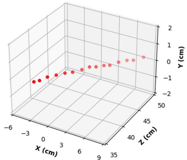
Fig. 4c The trajectory of the object when the camera makes an angle of 45° to the direction of motion
