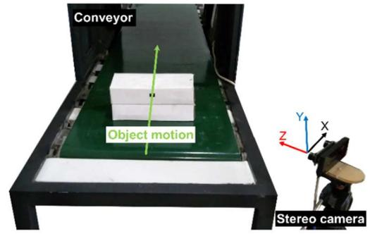
Fig. 2b Angle-looking velocity measurement
