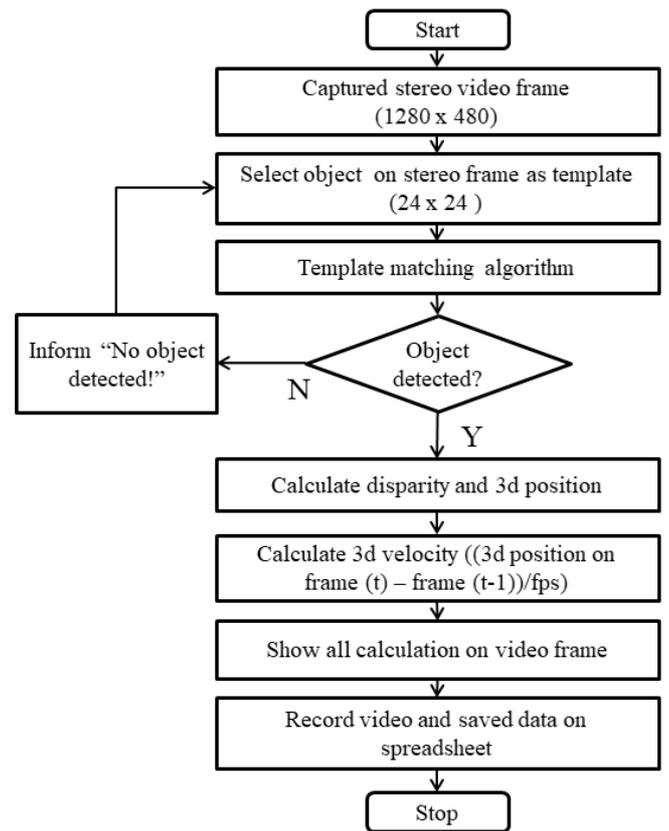
Fig. 1 System performance flowchart
