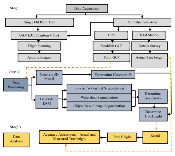
Fig. 1 Research Methodology in Determination Tree Height using UAV Images
