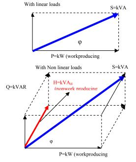
Fig. 1 Power factor relationship for Linear and Non-Linear loads
