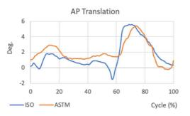
Fig. 2 Anterior Posterior Displacement in accordance with ISO142431 and ASTM F3141-17
