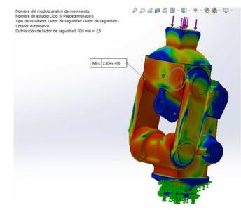
Fig. 18 Finite element simulation of the Streifeneder 3A20 knee joint
