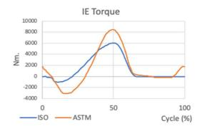
Fig. 5 Internal - external torque according to ISO142431 and ASTM F3141-17
