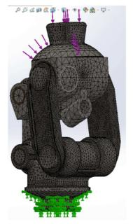
Fig. 17 Streifeneder 3A20 knee joint digitization
