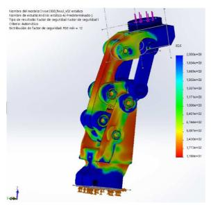
Fig. 15 Finite element simulation of the Ossur 2000 knee joint.
