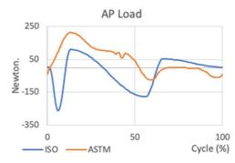
Fig. 6 Anterior-posterior loading under ISO142431 and ASTM F3141-1
