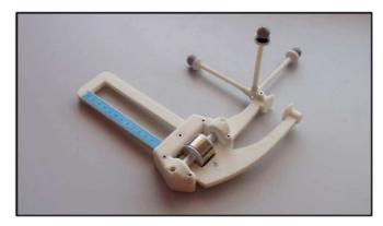
Fig. 9 Device for defining the flexion axis (KAD, Knee Alignment Device) [10].
