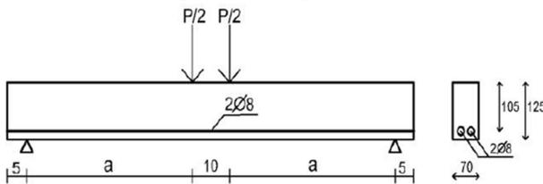
Fig. 2 Model of the beam specimen [34]
