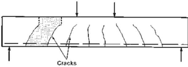
Fig. 1 Inclined cracks on beam [25]
