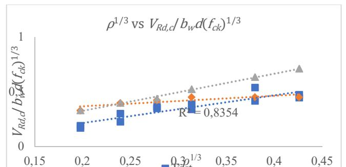
Fig. 4 Cube root of longitudinal reinforcement ratio vs non-dimensional ratio  $V_{Rd,c}/b_w d(f_{ck})^{1/3}$
