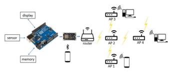
Fig. 4 Wireless engine monitoring can be accessed in a limited local area [26].
