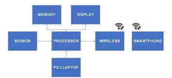
Fig. 3 General Design of Engine Monitoring Device That Uses A Wireless Connection [46]
