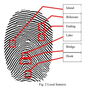
The local features that consider as most important and affected in fingerprint images are dot (or island), ending, bifurcation, hook, lake, bridge [7], as illustrated in fig. (2). From previous features, only two of them are originally used in fingerprint systems: ending and bifurcation [8].
