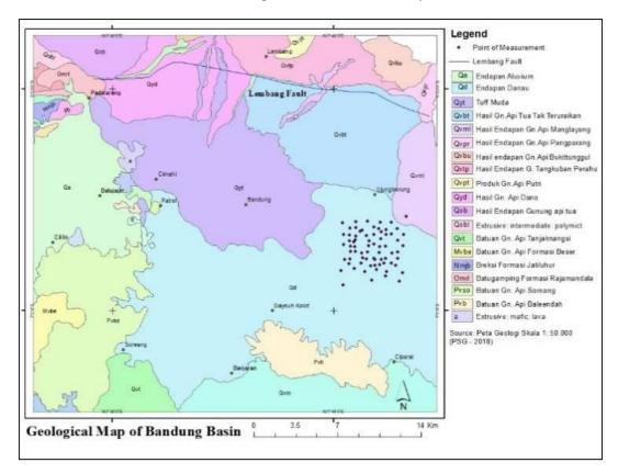
Fig. 3 Geology map of the Bandung basin is compiled and simplified from previously published maps [14]-[17]. The picture also shows the measurement location of microtremor (black dots).
