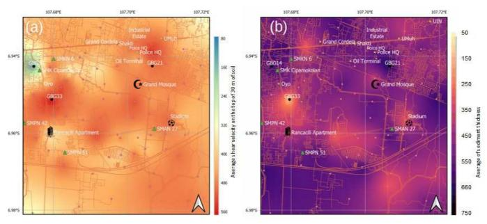
Fig. 6 Maps of (a) Vs30 and (b) sediment thickness (Z1.0) inferred from the inverted shear-wave velocity of Gedebage area. Figure 6a show the variation value of Vs30 in the study area between 80 m/s and 560 m/s and dominated by the value of Vs30 from 320 to 480. Only a small area has a value of 160 m/s and value of 560 m/s. Figure 6b show sediment thickness of study area ranging from 50 to 750 m.
