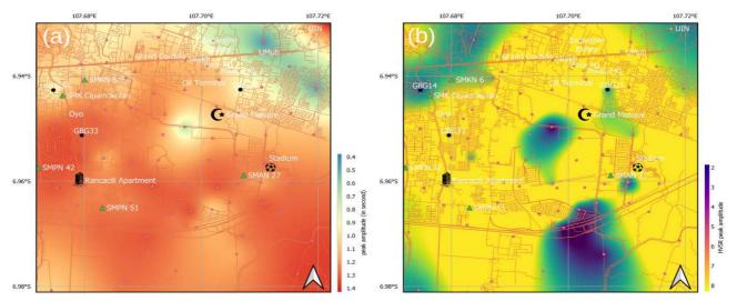
Fig. 4 Maps of HVSR (4a) peak period and (4b) peak amplitude. The figure 4a shows that peak period from 0.4 to 1.4 second mean medium and soft rock, mainly in the range of 1.2 - 1.4 second. Figure 4b shows the peak amplitude of the study area that mostly in the range 7 - 8; they reach lower in some areas.
