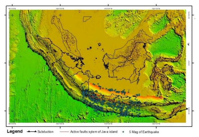
Fig. 2 Regional geology of Java island shows the main source of earthquake: megathrust in the south of Java and active faults in the land. [9].
