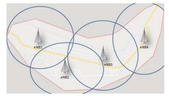
Fig. 12 The scheme of the LTE network in Muynak (with the geographical location of base stations)
