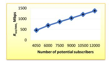
Fig. 11 The graph of the dependence of  $R_{\mbox{tot/HML}}$  on the number of potential subscribers
