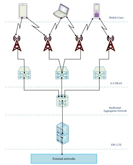
Fig. 13 The scheme of the LTE network in Muynak (with the geographical location of base stations)
