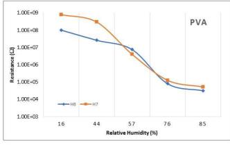
Fig. 10 Comparison of sensor resistance with PVA as the sensing layer
