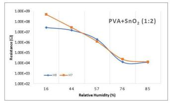
Fig. 12 Comparison of sensor resistance with PVA+SnO2 (1:2) as the sensing layer
