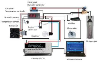
Fig. 5 Experimental setup for the measurement of relative humidity sensors
