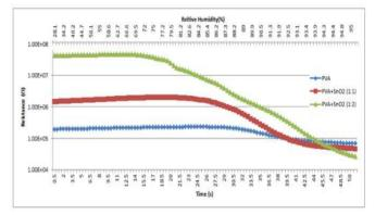
Fig. 8 Response time of the humidity sensors
