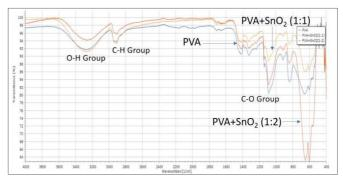
Fig. 2 FTIR test results of the PVA based sensitive layer
