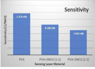
Fig. 7 The sensitivity of the sensing layers
