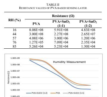
Fig. 6 The effect of SnO2 concentration on-resistance of the sensing layer
