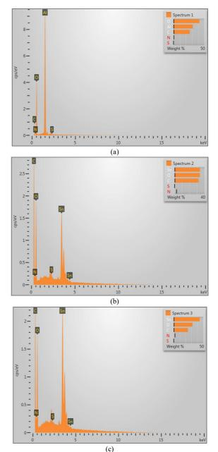
Fig. 4 EDS test results of the sensing layer (a). PVA, (b). PVA+SnO<sub>2</sub> (1:1), and (c). PVA+SnO<sub>2</sub> (1:2)
