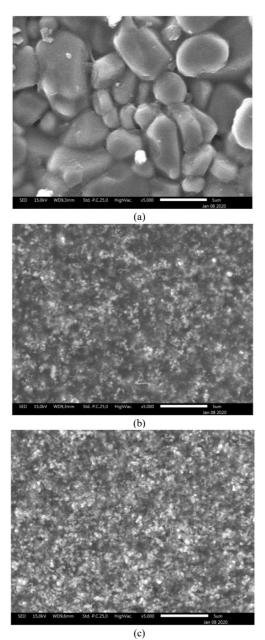
Fig. 3 SEM images of the sensing layer (a). PVA, (b).  $PVA+SnO_2$  (1:1), and (c).  $PVA+SnO_2$  (1:2)
