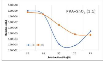
Fig. 11 Comparison of sensor resistance with PVA+SnO2 (1:1) as the sensing layer
