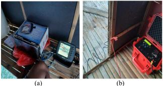
Fig. 1 Device's picture. A) fish-finder, B) S-FAD
