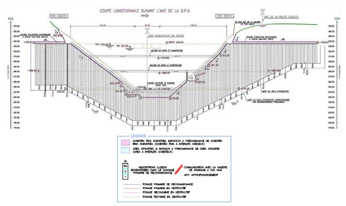
Fig. 3 Conception of the grout curtain of Tiddas dam
