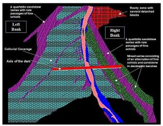
Fig. 1 The main features of the geology of the Tiddas dam
