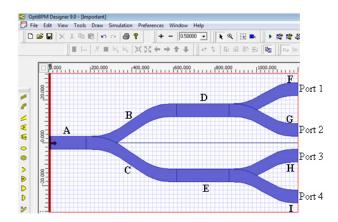
Fig. 1 Schematic view of 1×4 optical power Splitter
