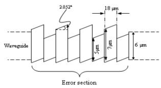
Fig. 2 Schematic representation of error section
