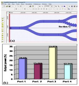
Fig. 10 Is the same as figure 4 but the fabrication error is considered in section G
