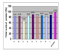
Fig. 13 Total output power of 1×4 optical power splitter considering fabrication errors in each section.
