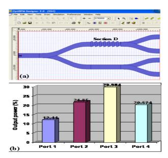
Fig. 7 Is the same as figure 4 but the fabrication error is considered in section D.
