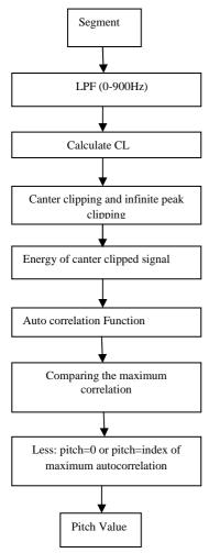
Fig. 2 Block diagram of PDA using modified autocorrelation method
