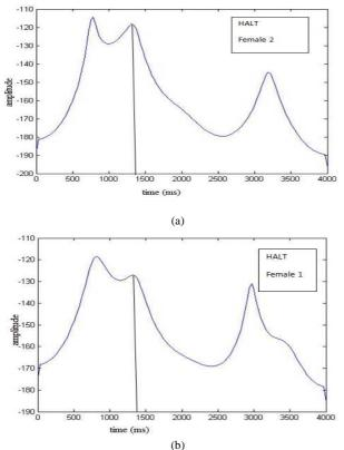
Fig. 7 (a) PSD of 'halt' for female 1 and (b) PSD of 'halt' for female 2 indicating 2nd formant
