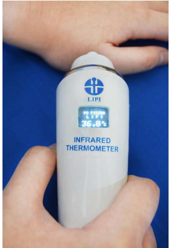
Fig. 1 A calibrated our own made infrared thermometer was used around 1 cm from the target. Although other general infrared thermometers are not interchangeable [21], this instrument can be used to measure equally well the ear canal and overhead
