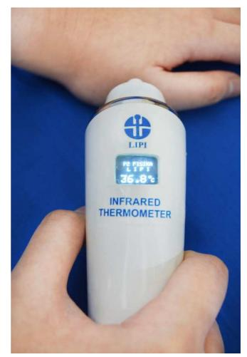
Fig. 1 A calibrated our own made infrared thermometer was used around 1 cm from the target. Although other general infrared thermometers are not interchangeable [21], this instrument can be used to measure equally well the ear canal and overhead
