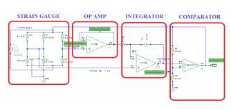
Fig. 1 Schematic of SFC
