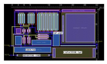
Fig. 7: Monolithic Integrator layout
