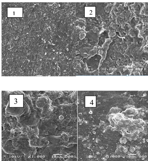
Fig. 6 SEM images of membrane composites with various compositions of PVDF/NH<sub>4</sub>Cl/NPM/AC+TiO<sub>2</sub> (1) 15/0/85/0, (2) 13/1/85/1, (3) 11/2/85/2, (4) 9/3/85/3
