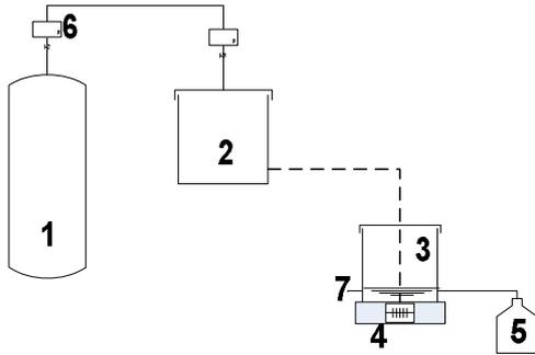
Fig. 1 PVDF Membrane system (1)  $N_2$  gas cylinder, (2) Feed tank, (3) Dead-end stirred cell (4) Magnetic stirrer (5) Beaker glass (6) Pressure gauge (7) Membrane composite
