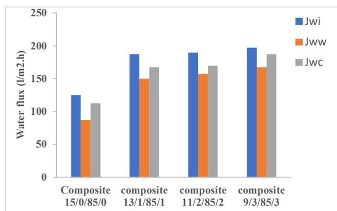
Fig. 3 The permeability flux of composite membrane used in this work
