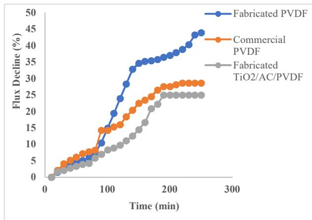
Fig. 5 The comparison of flux decline percentage among commercial PVDF, fabricated PVDF, and fabricated TiO<sub>2</sub>/AC/PVDF membranes
