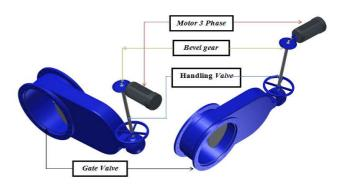
Fig. 2 Designing of automatic rotation valve
