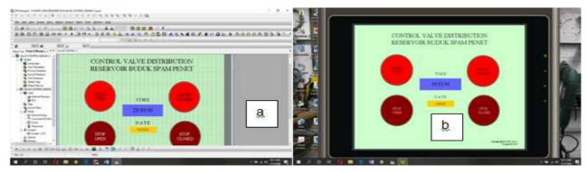
Fig. 7 Display Application for Making Ladder Diagrams (a) and Display Human Machine Interface (HMI) when running (b)
