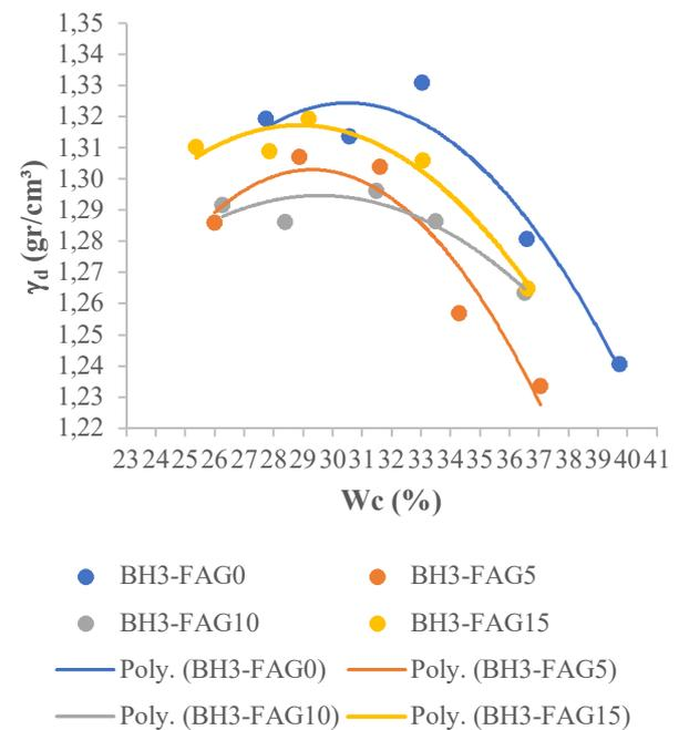
Fig. 3 Compaction Curve of BH3 soil at different FAG additions
