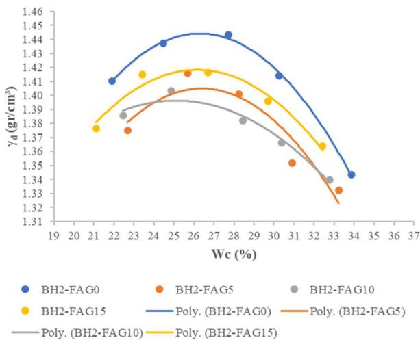
Fig. 2 Compaction Curve of BH2 soil at different FAG additions
