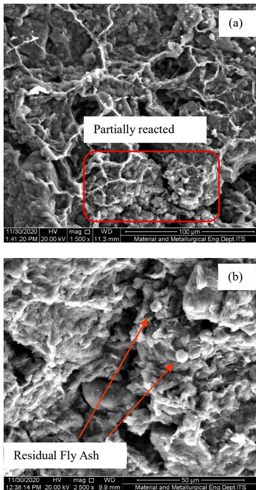
Fig. 9 The SEM images of 5% wt. (a) and 15% wt. of FAG addition
