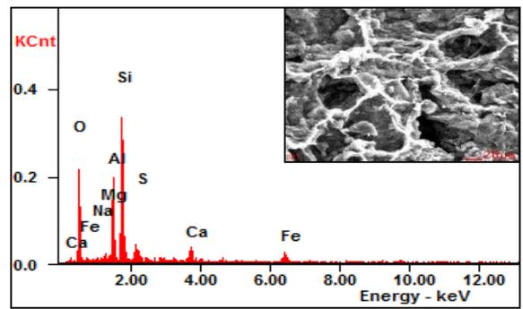
Fig. 7 The result of SEM-EDX of BH2 Soil
