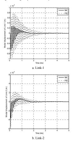
Figure 4: Deflection response of the system without payload.
