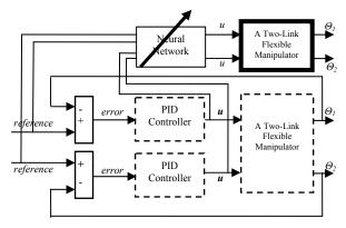
Figure 2: The structure of the neural network controller.
