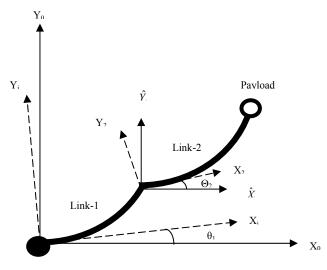
Figure 1: Structure of a two-link flexible manipulator.
