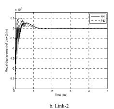
Figure 7: Deflection responses of the system with load 0.05 kg.
