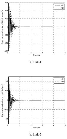
Figure 8: End-point acceleration of the system with load 0.05 kg.
