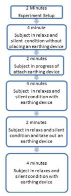
Fig. 3 Experiment process flow for an earthing application
