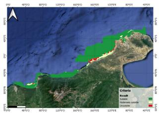
Fig. 10 Suitability map to the installation of a buoy-type WSN in the upwelling zone of the southern Caribbean Sea
