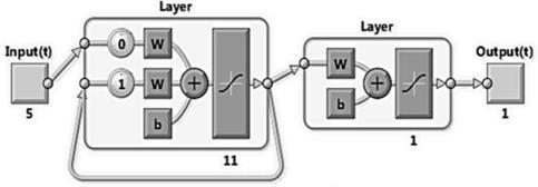
Fig. 2 The structure of RNN
