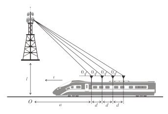
Fig. 2 The proposed array antenna-assisted DSC for FRMCS.
