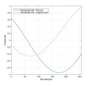
Fig. 10 The change of the channels at  $f_d T_s = 0.5$  with blocklength 256.
