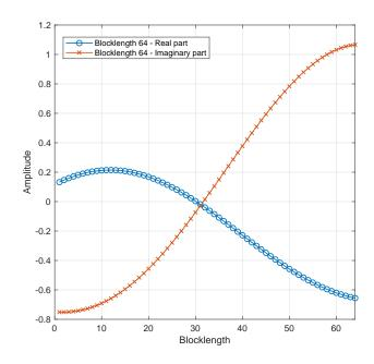
Fig. 9 The change of channels at  $f_d T_s = 0.5$  with blocklength 64.
