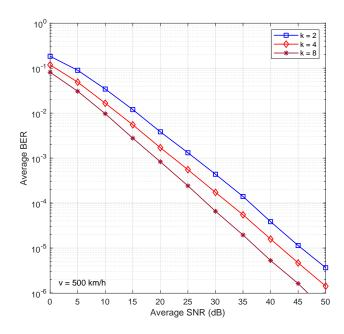
Fig. 6 The BER performances of FRMCS with K array-antenna element.
