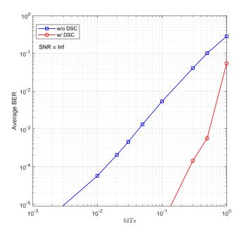
Fig. 7 The BER performances of FRMCS with and without DSC at different  $f_d T_s.$
