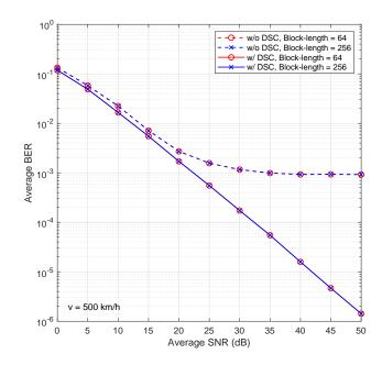
Fig. 8 Performances of FRMCS with and without DSC showing that the performance is not affected by the blocklength due to the normalized Doppler.
