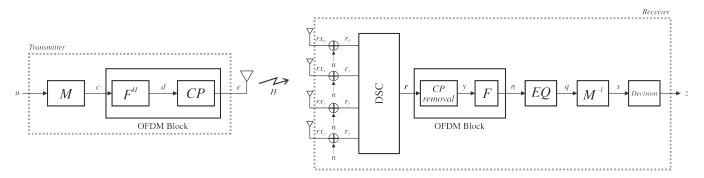
Fig. 1 Transmission structure of FRMCS using the proposed DSC.
