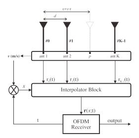
Fig. 3 The detailed struture of the proposed array antenna-assisted DSC.
