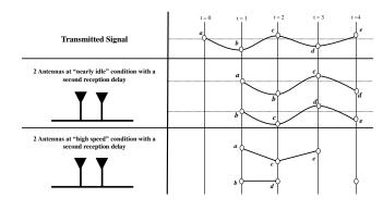
Fig. 4 Effect of Doppler spread experienced by each antenna element.
