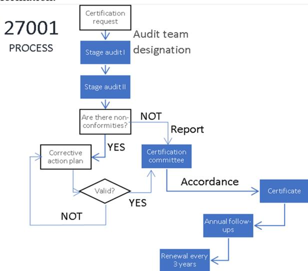
Fig. 3 Certification process of the International Organization for Standardization (ISO)/International Electrotechnical Commission (IEC) 27001
