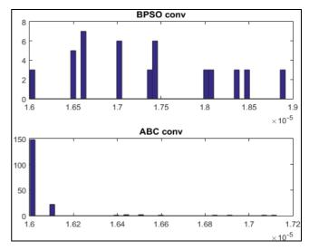
Fig. 2 BABC and BPSO convergence histogram for the FRA NARX model. BABC managed to consistently discover the best solution  $(1.60 \times 10^{-5})$  even when given different test parameters. The BPSO results were more distributed, discovering many different model structures resulting in various fitness values
