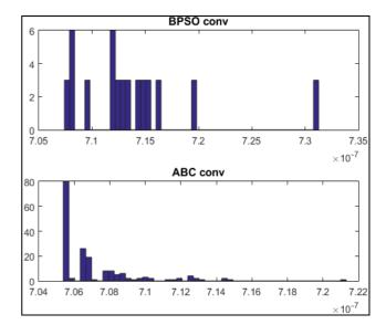
Fig. 4 BABC and BPSO convergence histogram for the MA NARX model. BABC managed to consistently discover the best solution  $(7.05 \times 10^{-7})$  even when given different test parameters. The BPSO results were more distributed, discovering many different model structures resulting in various fitness values
