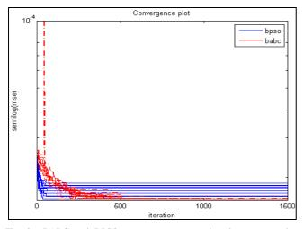
Fig. 3 BABC and BPSO convergence across iterations over various parameter combinations. BABC solutions are more gradual compared to BPSO, but BABC has the ability to explore in a more in-depth manner resulting in a much better fitness relative to BPSO
